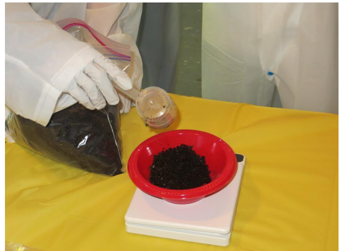
Weighing the soil for the turbidity tests.
