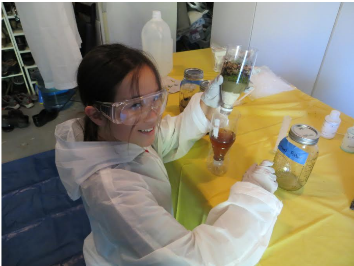
Filtering water through a gravel, sand, and cheesecloth filter.
